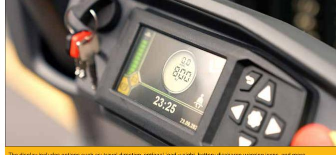
The display includes options such as: travel direction, optional load weight, battery discharge warning icons, and more.
